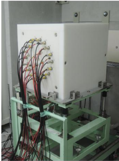
Fig. 2. (Color online) The experimental setup of the flat-response neutron detector.
